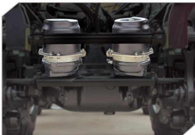
Elevated brake chambers
