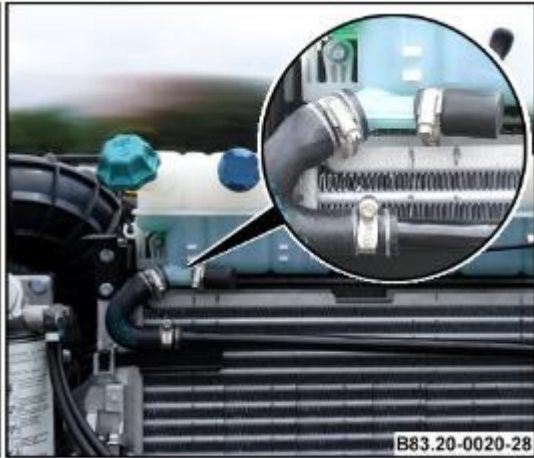
Return of the heating coolant
