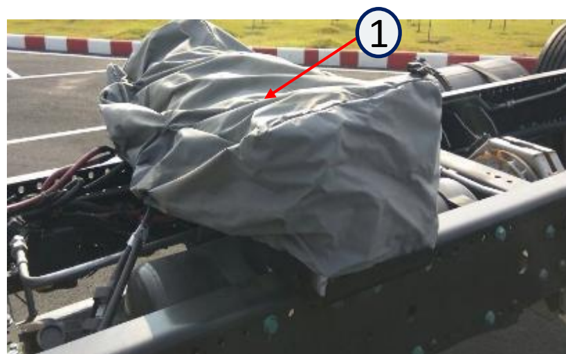
Battery compartment B54.10-0009-02 Electronic relays (arrows) 1 Plastic cover for battery protection 2 Protection removed from batteries
