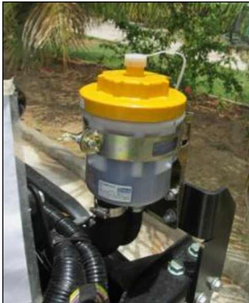
Power steering oil tank
